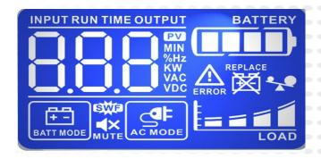
LCD display indicates input voltage, output voltage, load level, battery capacity, operation mode, and alarm conditions.
