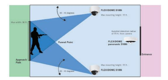
Install the system at entrances, high traffic funnel points, and approach paths up to 30-feet wide to provide early warning while remaining nearly transparent and frictionless as opposed to metal detection systems. This system consists of the following components:
