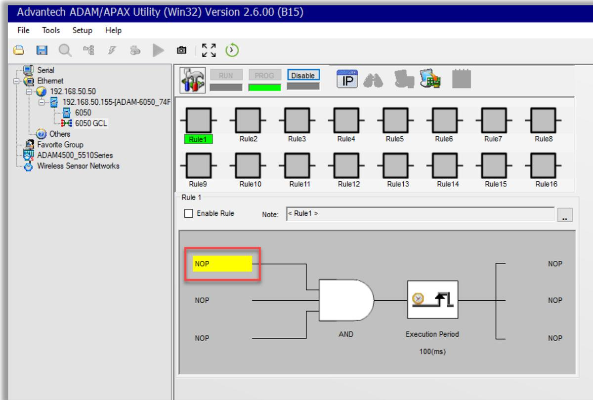
Step 6: In the pop-up window, set the Mode to “DI”, set the input channel you want the rule to apply to, and set the Condition to “False”. Remember, DI’s are numbered 0-11. In this example we are using DI 1. Click OK.
