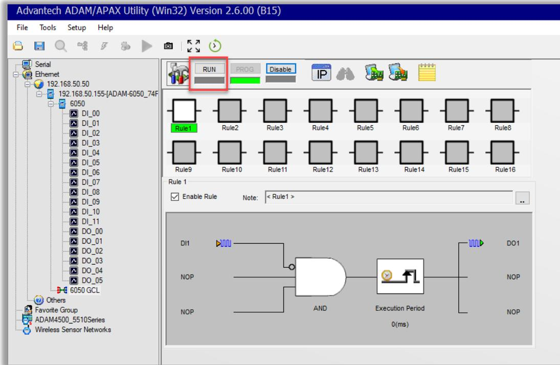
Step 14: Verify running state. By default, monitoring will be enabled which is represented by yellow circles. When you short the associated Digital Input, you will see the yellow circles progress to the right. You should check continuity with a multi-meter on the Digital Output you associated to make sure you are getting a closer before you connect to the endpoint device. This completes the configuration to have the output follow the input state. No further action required.
