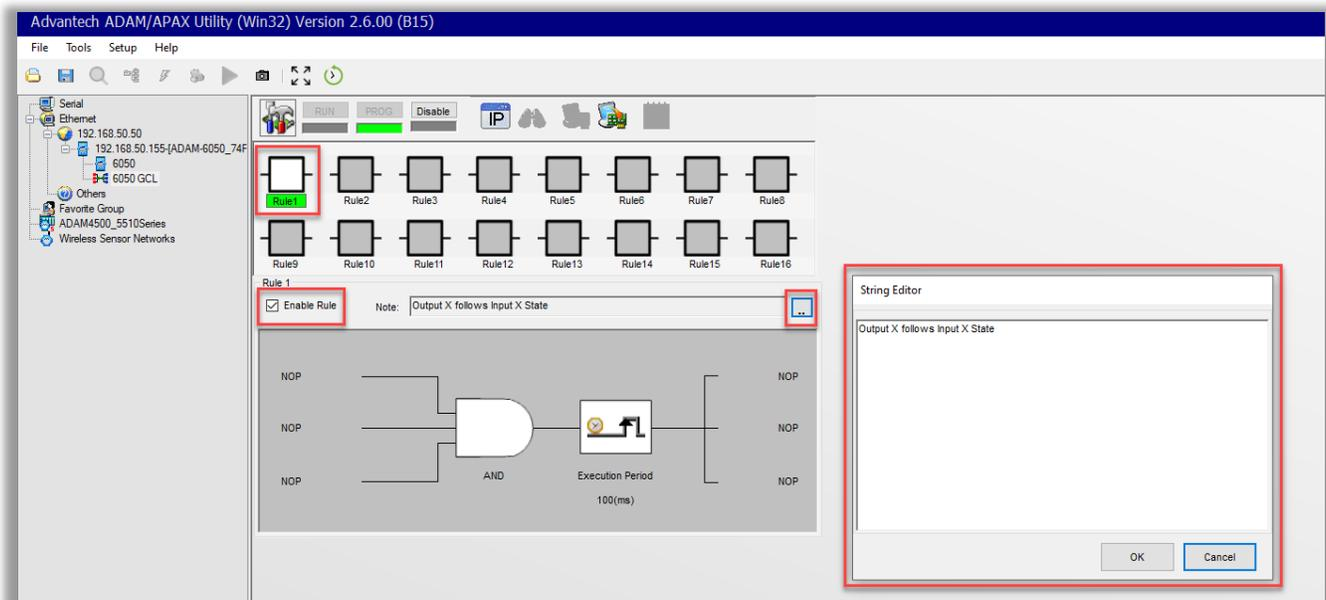
Step 4: Highlight the top “NOP” option in the Input Condition Stage area.
