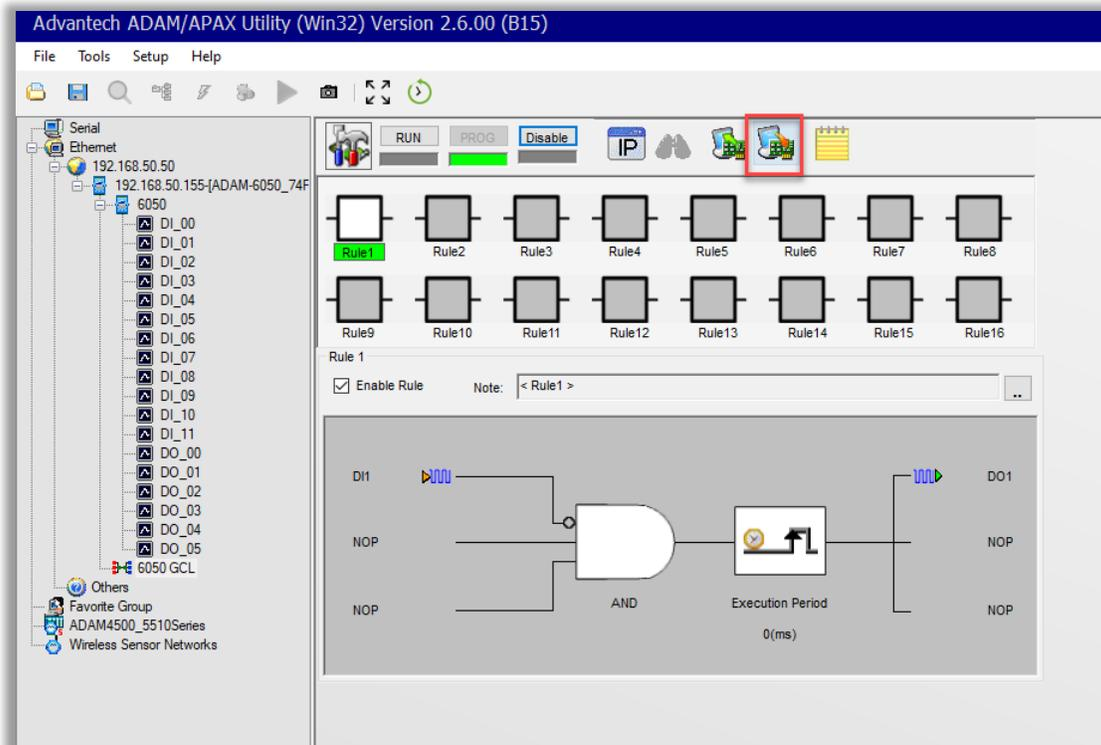
Step 13: Click on RUN to have the rule start and continuously run.
