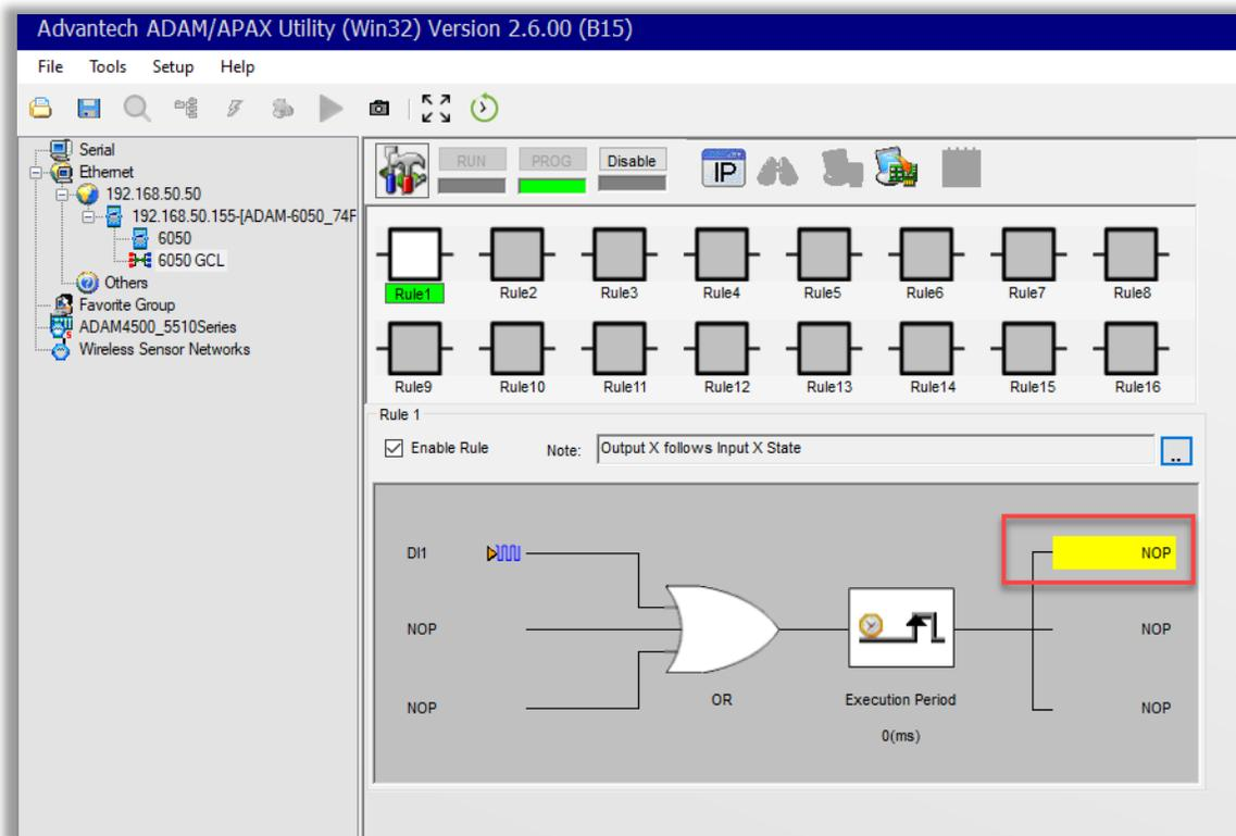
Step 11: Set the Operation Type to DO (Digital Output), and assign the channel (output) that you want the rule associated to. Remember, the ADAM 6050 has six Digital Outputs that are numbered 0-5. In this example we are using DO 1.
